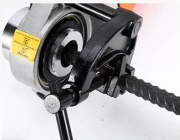
3. The clamp is fixed on the machine
