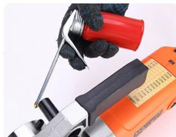
6. Lubrication operation for rigid tubing threaded connection
