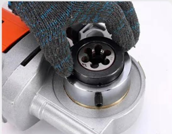
1. Install the round die as shown in the diagram above
