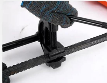
2. Fixture to secure threaded steel bars
